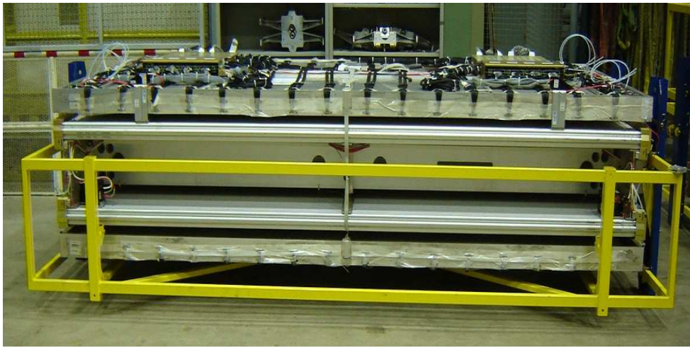
Figure 6.1: Assembled BML muon station before installation on the apparatus. BM stations are made by two RPC planes with the MDT chamber 'sandwiched' between.
